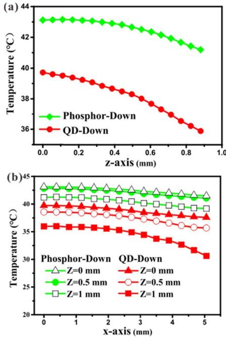
Fig. 10. Simulated temperature distributions of the QD layer along (a) *z*-axis and (b) *x*-axis.
