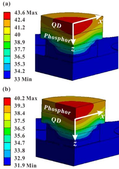
Fig. 9. Simulated temperature fields at the cross sections of the bw-LEDs based on (a) red-phosphor-down and (b) green-QD-down SPSs at an injection current of 100 mA.
