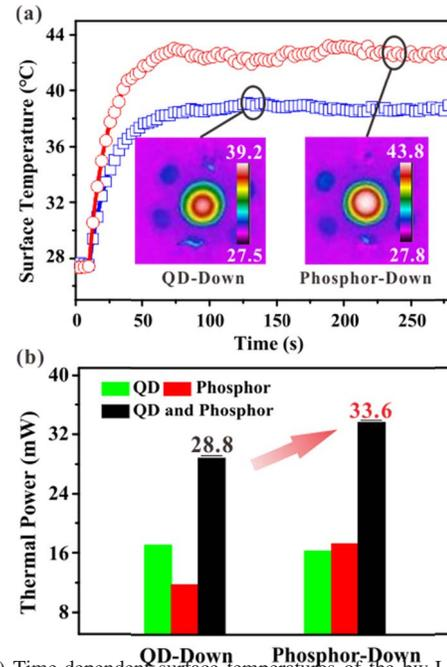
Fig. 7. (a) Time-dependent surface temperatures of the bw-LEDs based on different SPSs at the injection current of 100 mA; the insets are their steady thermal images, and the unit is degree Celsius. (b) Thermal powers generated by the conversion layers in different SPSs.
