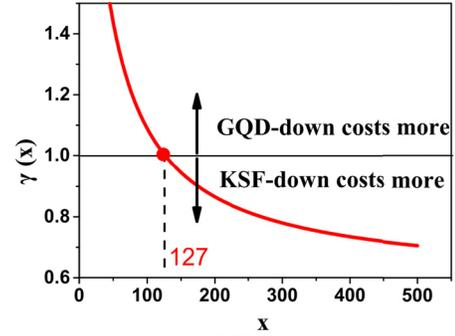
Fig. 6. Cost ratio curve of the bw-LEDs based on the green-QD-down SPS and red-phosphor-down SPS.
