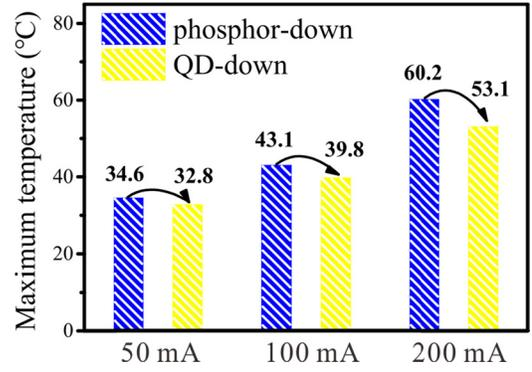
Fig. 11. Simulated current-dependent maximum temperatures of QD layer in bw-LEDs based on different SPSs at the injection current of 50, 100, and 200 mA.
