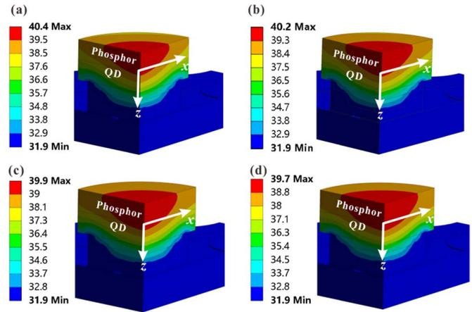
Fig. 8. Simulated temperature fields at the cross sections of the bw-LEDs based on the green-QD-down SPSs at an injection current of 100 mA with different thermal conductivities of red-phosphor layer. (a) 0.3 W/m·K. (b) 0.35 W/m·K. (c) 0.45 W/m·K. (d) 0.55 W/m·K.
