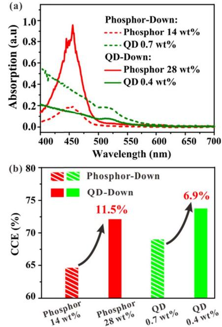
Fig. 5. (a) Absorbance spectra and (b) CCE of the conversion layers in the green-QD-down and red-phosphor-down SPSs.
