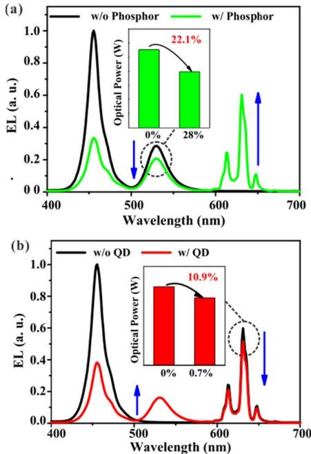
Fig. 4. EL spectra of the LED devices based on (a) green-QD-down SPS with and without the red-phosphor layer and (b) red-phosphor-down SPS with and without the green-QD layer.
