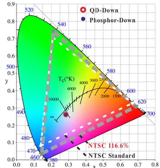
Fig. 2. CIE 1931 color coordinates of the bw-LEDs with the green-QD-down and red-phosphor-down SPSs, at a typical injection current of 100 mA.
