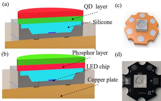
Fig. 1. Schematics of the bw-LEDs with (a) green-QD-down SPS and (b) red-phosphor-down SPSs. (c) Schematic of blank LED. (d) Real photograph of blank LED.
