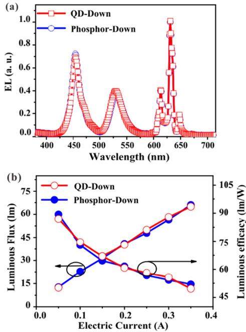
Fig. 3. (a) EL spectra of the bw-LEDs with the green-QD-down and red-phosphor-down SPSs, at a typical injection current of 100 mA. (b) Injection-current-dependent luminous flux and efficacy of the devices.
