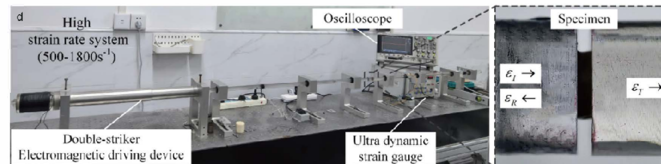
Physical diagram of the Double-striker electromagnetic driving Long Split Hopkinson Pressure Bar (LSHPB) system
