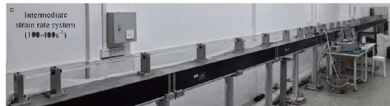
Physical diagram of the Double-striker electromagnetic driving Long Split Hopkinson Pressure Bar (LSHPB) system
